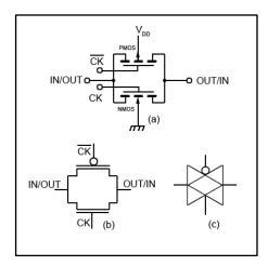
**4.5**Static Energy Recovery Full Adder (SERF):In this type of adder, the energy recovering logic reuses charge and therefore consumes less power than non-energy recovering logic. The circuit consists of two XNORs realized by 4 transistors. Sum is generated from the output of the second stage XNOR circuit. The C<sub>out</sub> can be
