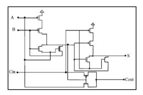
**4.6** Gate Diffusion Input: The circuit operation of GDI based full adders, is exactly the same as that of previous SERF module. Sum bit is obtained from the output of the second stage of XOR circuit while carry bit (C<sub>out</sub>) is calculated by B and C<sub>in</sub> controlled by (A XNOR B).
