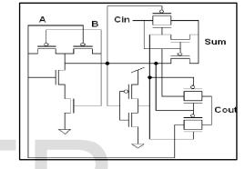
**4.4**CMOS Transmission Gate (TG): Transmission gate logic circuit is a special kind of pass-transistor logic circuit. It is built by connecting a PMOS transistor and a NMOS transistor in parallel, which are controlled by complimentary control signals.
